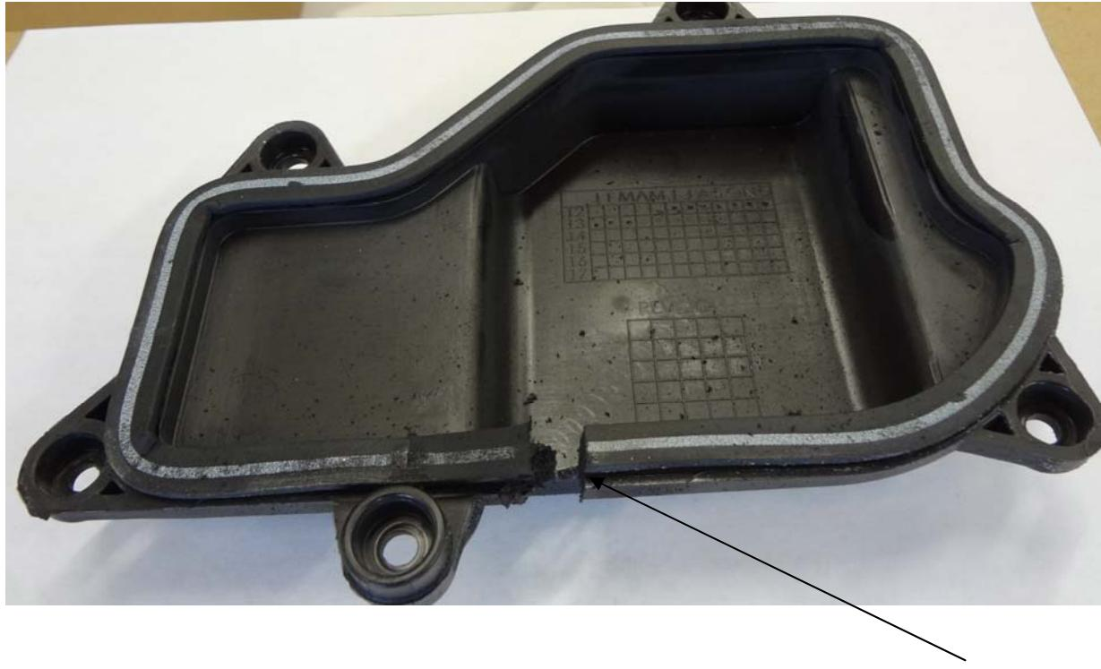
Cut a groove (3/8" x 3/8") in the cover of the light housing. After installation of adapter 800077 run all wires through the cutout. **Silicone** the groove after installation of the cover to the light housing.
